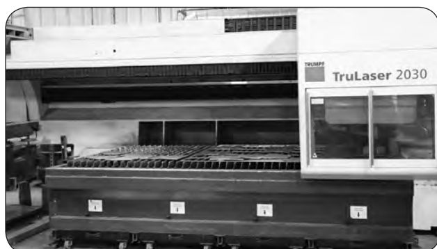
Diemo's laser cuts sheet metal.
