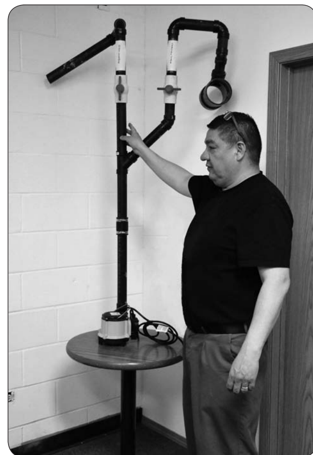
Peguis' emergency co-ordinator William Sutherland demonstrated the simplicity of the diverter attached to a pressurized sump pump.
