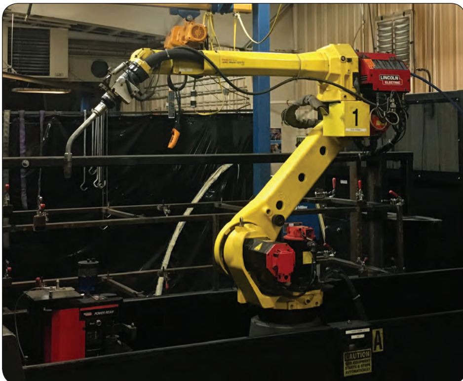
Vidir's robotic welder allows for precision welds.
