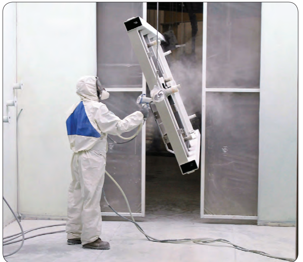
EXPRESS PHOTOS COURTESY OF VIDIR VERTICAL STORAGE SOLUTIONS A painter powder coats one of the custom-ordered units.
