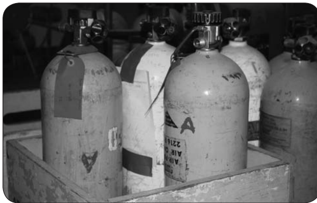
The station has about 20 obsolete breathing apparatuses, which lack CSA approval. They are also significantly heavier than approved models, creating added weight for firefighters.
