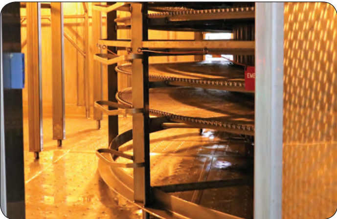
14. FFMC has flash freezers and a massive on-site cold storage that can hold about 1 million pounds of fish, which includes mullet, carp, sauger, perch and goldeye. The spiral freezer shown here has a moving belt on which fish is placed and rotates from bottom to top. As the fish turns, it's blasted with cold air, resulting in a perfectly frozen product.
