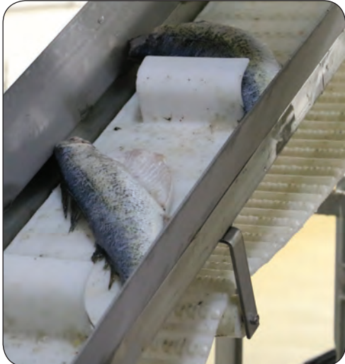
5. Once sorted by size, the fish is packed either whole in waxed food-grade cardboard boxes containing sterile ice or sent to the filleting line. The pickerel shown here are heading up a conveyor belt to have their scales removed before filleting.
