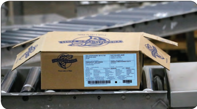
16. Fresh or frozen fish destined for domestic, U.S. and international markets is packed by machine in food-grade boxes. Each box is labelled and barcoded, identifying species, fish shed, lake, lot number and product code. "We track all the fish and that information stays in our system," said Bergunder. "With the label, we're able to trace the fish back to the shed. For recalls and food safety, it's critical."
