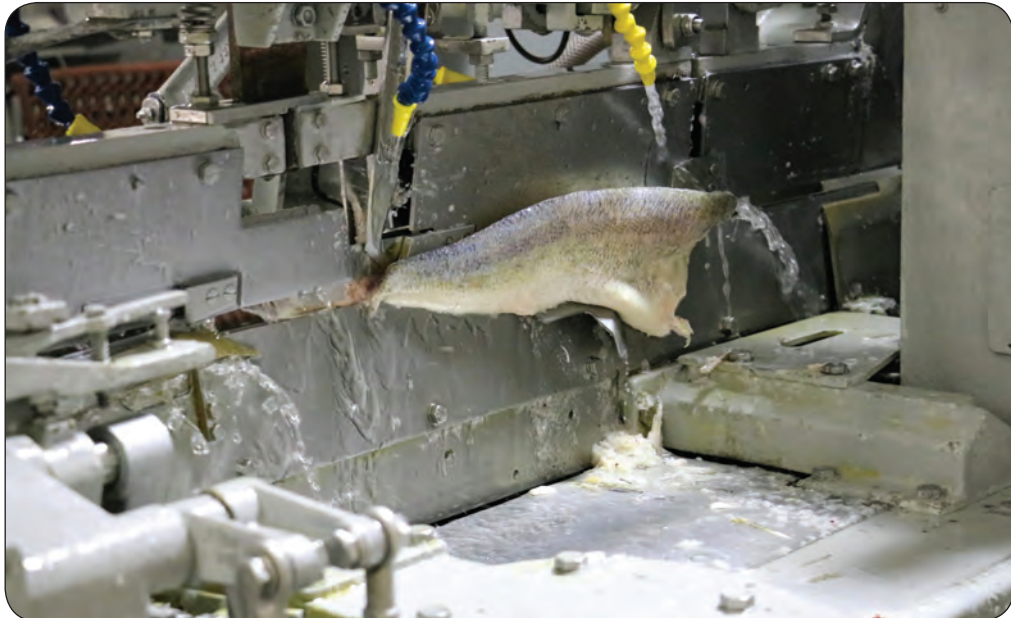
7. Pickerel is moved at a steady pace through a filleting machine and sliced in two by industrial-sized knives. The plant has eight lines and its fastest machine can cut 120 pounds of whole fish a minute.
