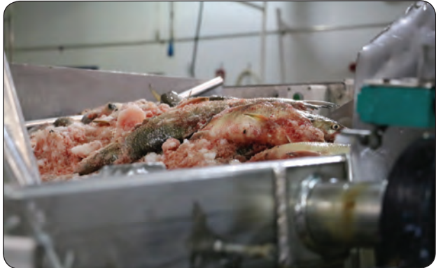
4. Before fish is sold whole or processed into fillets, FFMC sorts them by size into small, medium, large and jumbo. The fish are whisked through a measuring machine with a flapper that diverts them into clean totes. Sorting fish by size before they're run through the filleting machines improves plant efficiencies in that processing does not have to be halted to adjust the size and speed of the automated filleting blades.
