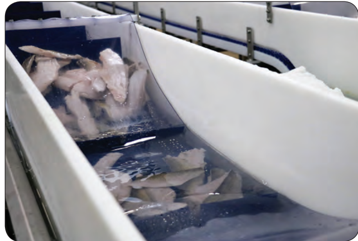
15. Fillets produced for the frozen market are sent through a glazing machine, which coats them with a thin film of icy water to prevent dehydration and freezer burn. FFMC's marketing strategy is focused on selling as much fresh fish as it can, said Bergunder, but the fresh market is finite.
