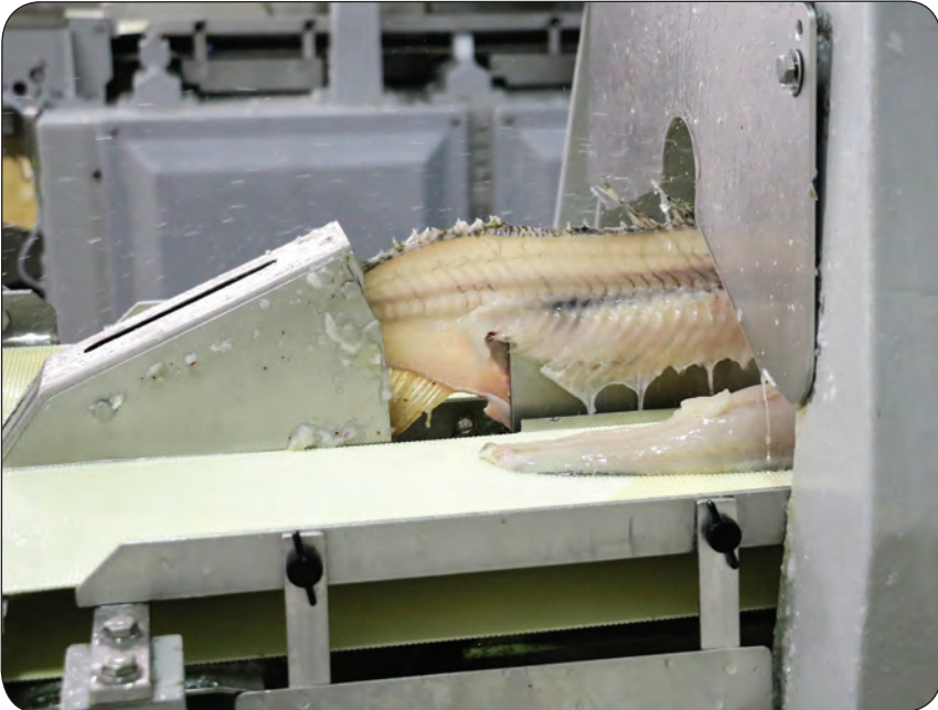
8. Sounding like a cross between a sawmill and an automatic car wash, the filleting machine removes the ribs and backbone after the fish is cut.
