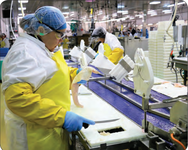
9. An employee checks each fillet cut by the machine and trims away excess. Freshwater employs over 180 full-time production staff, and those working the lines process about 25 to 30 fish a minute. Before they're allowed to enter the plant, staff must wash and disinfect their hands at a cleaning station and don smocks, aprons, gloves, safety glasses and steel-toed rubber boots. Hair must be secured under a hair net.
