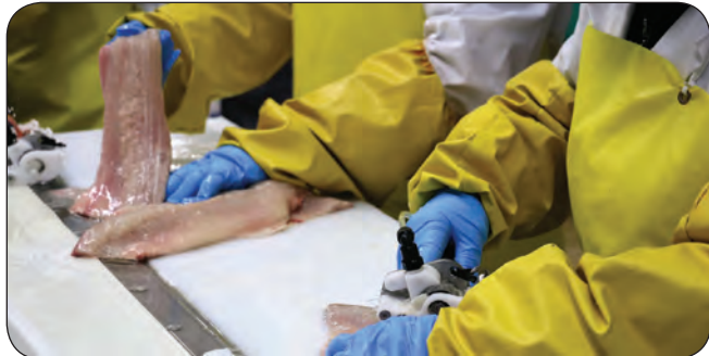
10. Employees on the pin-bone line check whitefish fillets for small bones, removing them with an electric de-boner and tweezers. Quality assurance standards are high; fillets containing more than one or two bones are unacceptable. FFMC's customers set standards that the plant must meet and will request inspections and audits. The plant is also a certified kosher facility with a rabbi on staff to inspect the fish.
